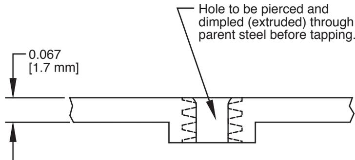
**Figure 3 – Extrusion to create (3) full threads of #12-24 (nm)**
