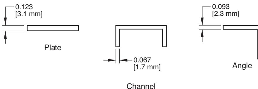
**Figure 1 – Rigidity of angle or channel versus plate**
