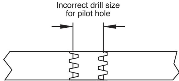
**Figure 5 – Full thread shall not fall below 65%**
