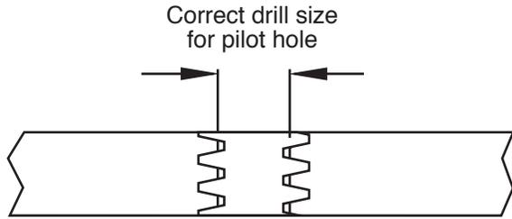
**Figure 4 – Maintain a minimum of 65% of full thread**
