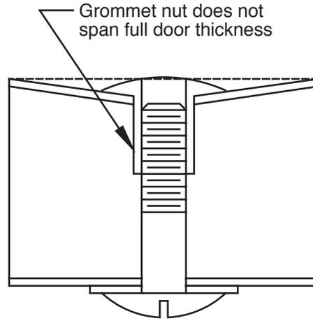
Figure 7 – Improper thru-bolting
